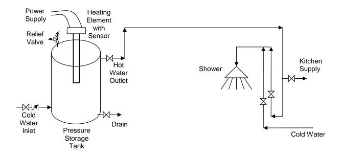
Figure 11: Simplified Flow Diagram of a Electric Domestic Hot Water System
