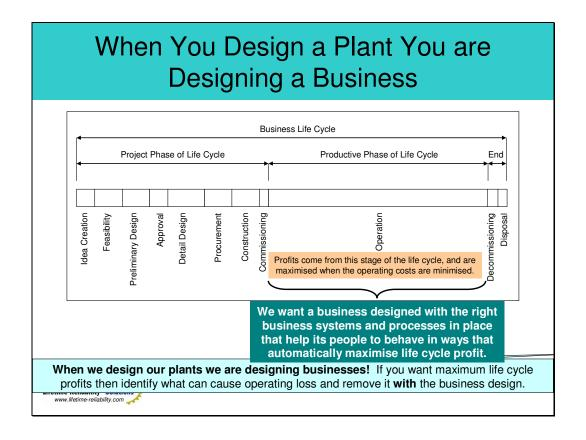
The plant and equipment used in an enterprise have a life cycle. It starts with the recognition of an opportunity, then progresses to feasibility and approval. If the idea is found worthwhile a full design is developed, plant and machinery are purchased, installed and put into operation. The vast majority of the life cycle is its operation and this continues until the plant and equipment are eventually decommissioned and disposed of.
