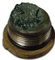
Caterpillar 785 Haul Truck Bearing Failure Magnetic Plug from 785 Haul Truck Left Rear Final Drive 4,412 operating hours on final drive 48,048 operating hours on truck ISO 21/20/18
