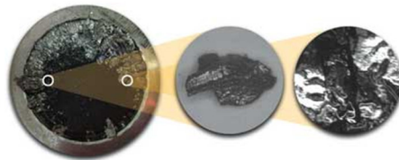
Magnetic drain plug used for warning of impending failure
