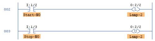
Activate the Start and Stop switches and ensure that the OTL and OTU output instructions are responding as outlined in your text. Once you have the lamp ON, could you turn it off if power was lost in the Stop Switch circuit?
